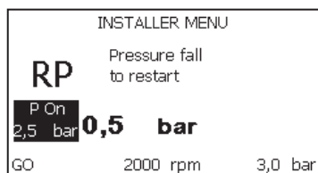
Figure 17: Setting the restart pressure
